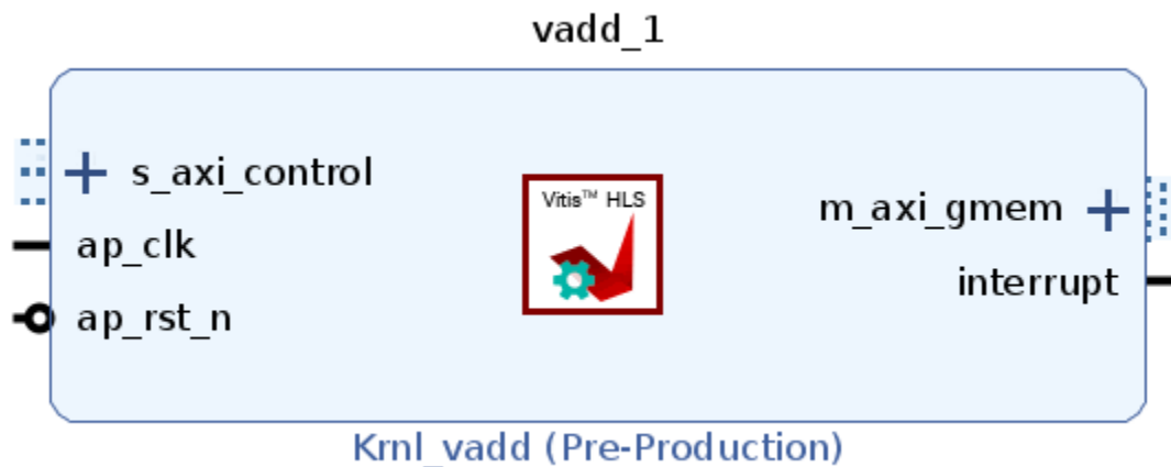
Figure 63: RTL Ports After Default Interface Synthesis
